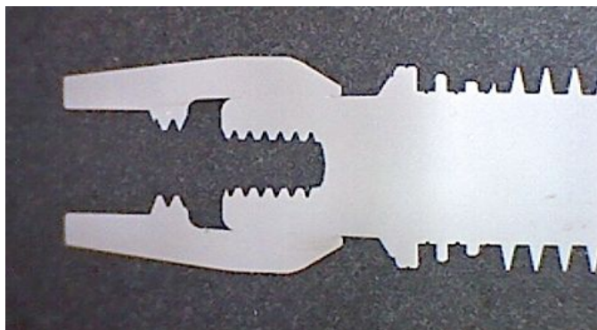
Figure 1, Cross section of the implant with the abutment inserted at 10X magnification
